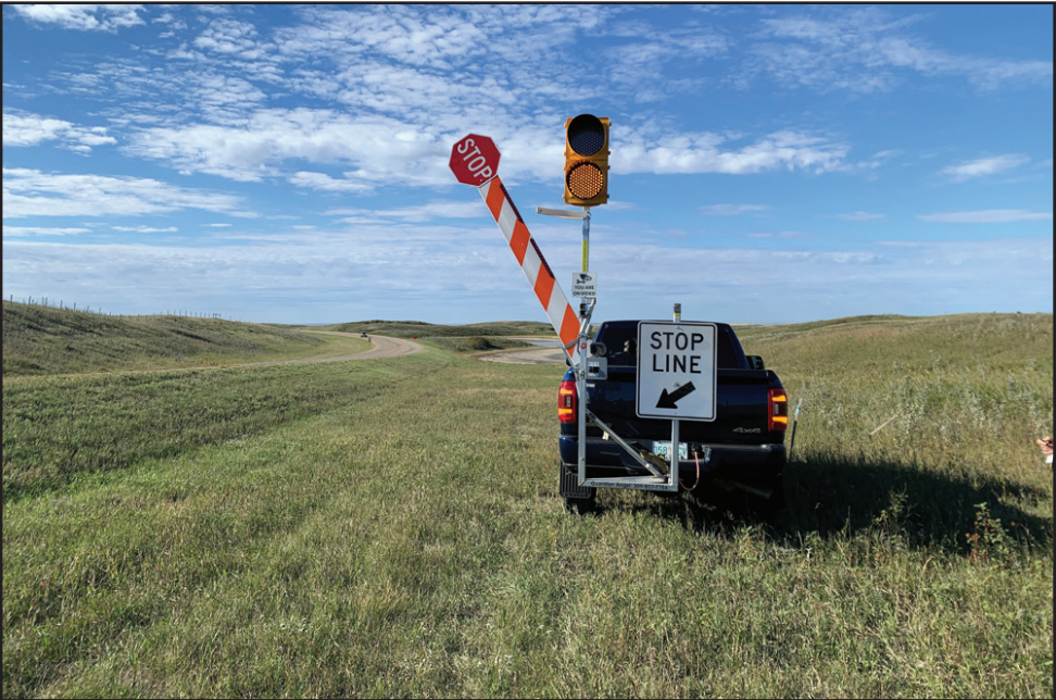
► Created by Watrous residents Kim and Donna Kreutzer, the Guardian Angel, a remote controlled automatic flagging assistance device is being tested in work zones in Saskatchewan. As part of a provincial pilot program, three sets of two of the
