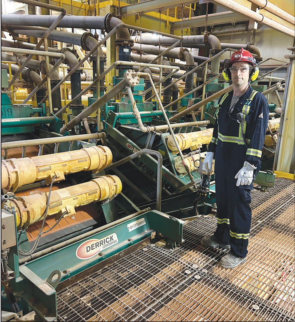
► Pictured: mill wet screening at Nutrien Lanigan with employee Jordan Lenuik, Mill Operator. photo courtesy Nutrien Lanigan
