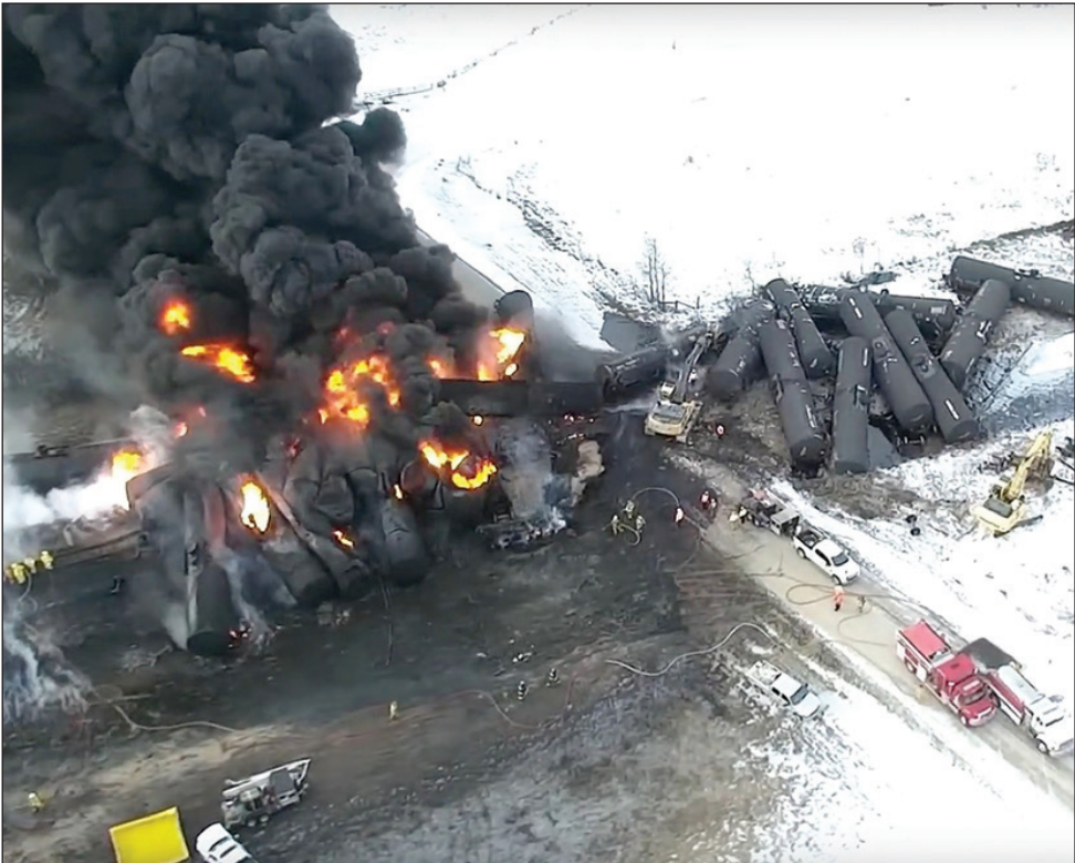
Following its investigation report, the Transportation Safety Board of Canada indicated the Dec. 9, 2019 derailment near Guernsey resulting in the release of 1.77 million litres of crude oil was the result of a gap in the rail. The south rail had likely failed under a previous train, causing an undetermined length of rail to break away and separate from the track, exposing the rail ends. - file photo
